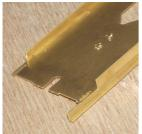
The next step is to bend up the narrower part of the brass to form the bottom of the solebar channel. To form this bend, press the flange against the work surface to bend it to about 45°, then place it against the edge of a rule and gently tap until the flange is at a right angle. When this is complete, solder can be run in from the back at the ends as reinforcement. The channel has now taken the form of a banana, but do not panic, nor try to straighten it. The next stage will do this for you.
