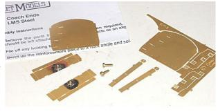
Repeat for the other side and end, ensuring that they are both the right way round, and then solder your two 'L' shaped pieces together. Now fold up the end steps (if present) to 90°, feed them through the slots in the end, and solder in place.
