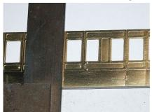
In these cases the first task is to score the door part lines on the lower section of the coach. This should be done using a small engineers square to align the score marks with the door part line etched in the upper section. The scoring itself should be done with a sharp scriber in two or three gentle passes to avoid distorting the side.
