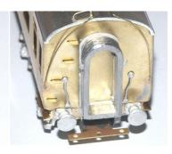
Corridor connections are provided as whitemetal castings. The bellows parts are soldered or glued together then fixed to the baseplate. The assembly is then fitted to the end of the coach with the baseplate against the coach end. In the case of bow ended coaches the baseplate is not used, the bellows section being attached directly to the coach ends.
