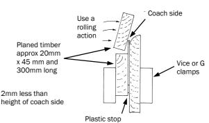
Once the start of the curve has been formed move the side up level with line B and repeat. It is best to overdo the curve then relax it with gentle finger pressure until it is a close match to the profile of the end etch.
